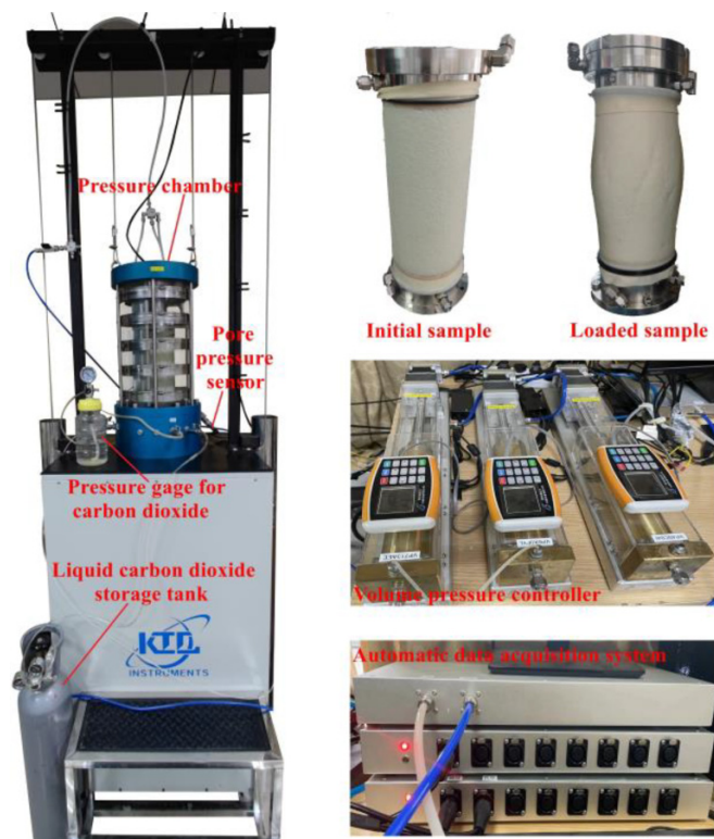
Fig. 4. Adopted test setup.
